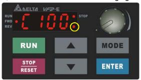
C. 10000~65535 display: It will only display the first 3 digits. The LED at the bottom-right corner and the single decimal point between the middle and the right-most numbers will light to indicate 100 times of the display value. For example, the actual value for the following figure is 100X100=10000.
