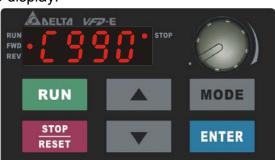
B. 1000 ~ 9999 display: It will only display the first 3 digits. The LED at the bottom-right corner will light to indicate 10 times of the display value. For example, the actual value for the following figure is 100X10=1000.
